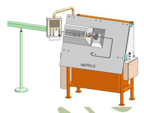
FULLY AUTOMATIC STIRRUP BENDER, WHERE THE FULL-LENGTH STOCK BARS ARE LOADED ONTO THE MACHINE, RECALLING THE PROGRAM THE MACHINE WILL CONTINUOUSLY FORM STIRRUPS WITH GOOD PRECISION AND SPEED.
